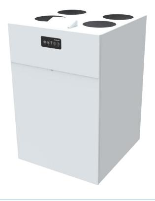
The HCV 500 is a highly efficient residential ventilation unit for houses, villas, and apartments of up to 450m<sup>2</sup> or more. It comes supplied as a packaged basic ventilation unit complete with built-in control panel, and are delivered with all parts necessary for wall installation. The HCV 500 is ideal for free wall installation with minimum 700mm space. A standard wall rail is supplied with all units.
